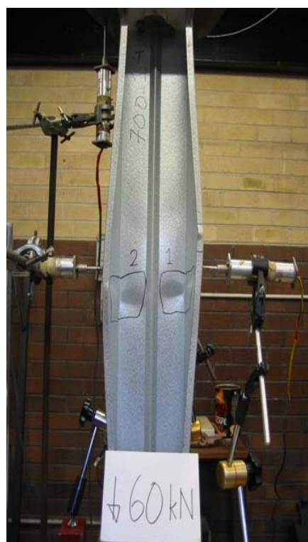
Fig. 6b Outward lip deflection failure mode of 700 mm column
