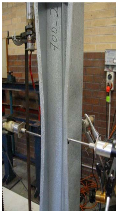
Fig. 6a Elastic local buckling occurring along flange with inward lip deflection of 700 mm column
