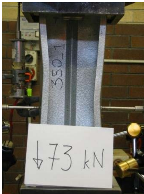
Fig. 5 Inelastic local buckling occurring in all flanges for 350 mm specimen
