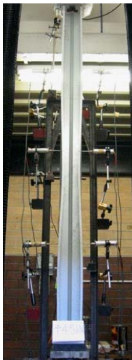
Fig. 9a Elastic distortion buckling with 3 buckle half-waves for 2000 mm column
