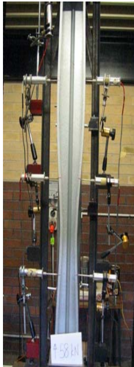
Fig. 8a Elastic distortion buckling with 2 buckle half-waves for 1300 mm column
