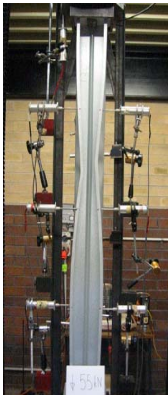
Fig. 8b Inward lip deflection failure mode of 1300 mm column
