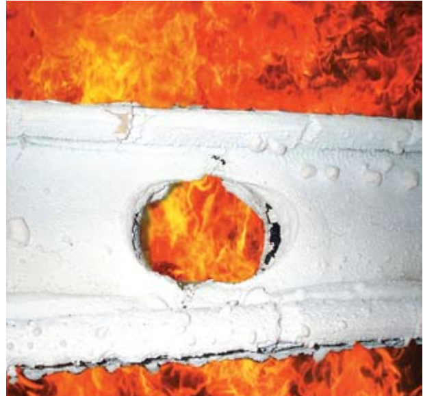
Fire test on intumescent coated Fabsec beam
