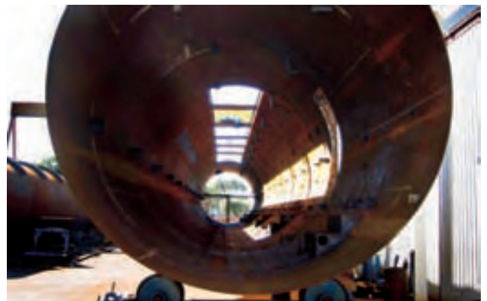
Right: The shuttle sections were fabricated with openings for the shuttle load chute, which runs the full length of the completed shuttle. All internal service and support bracketing was fitted and welded prior to completion saving valuable time on site.
