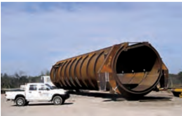
Left: Shuttle centre section weighing 52 tonne.
