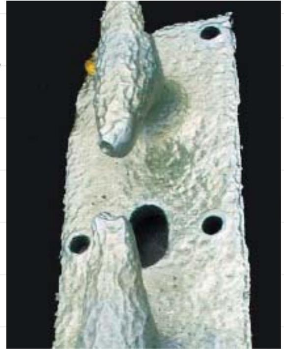
*This 50-year old cast marine bollard has been hot dip galvanized. Although it is badly pitted, the bollard was easily re-galvanized to restore its durability.*
