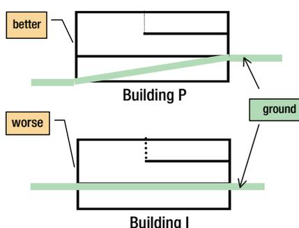
mezzanine level or (upper) ground level and their potential exposure to a fire, the two buildings are equivalent. In the case of occupants within the lowest level, it is argued that Building P is better than Building I, since direct egress to outside is available. It follows that Building P is at least as safe as Building I and therefore it is difficult to see why the requirements applicable to Building I should not apply to this building.
