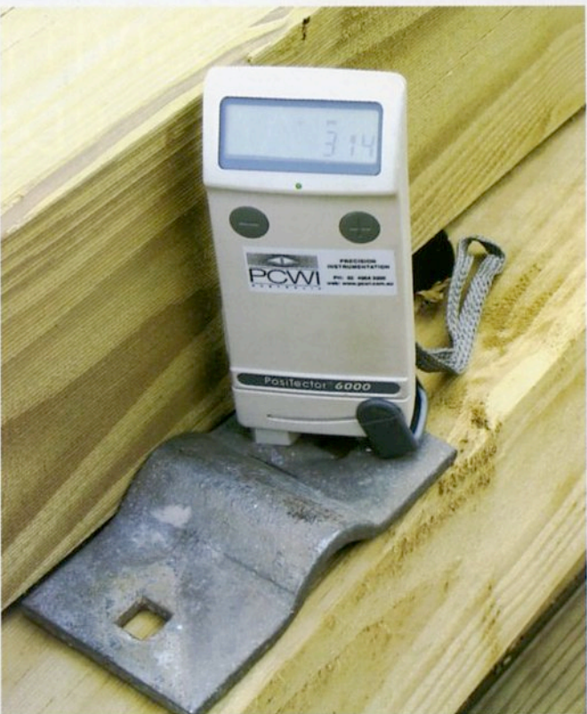
This galvanized bracket was salvaged from the Townsville to Charters Towers telegraph line built in 1888. Its galvanized coating exceeds 300 microns, indicating a service life expectancy of 1000 years.
