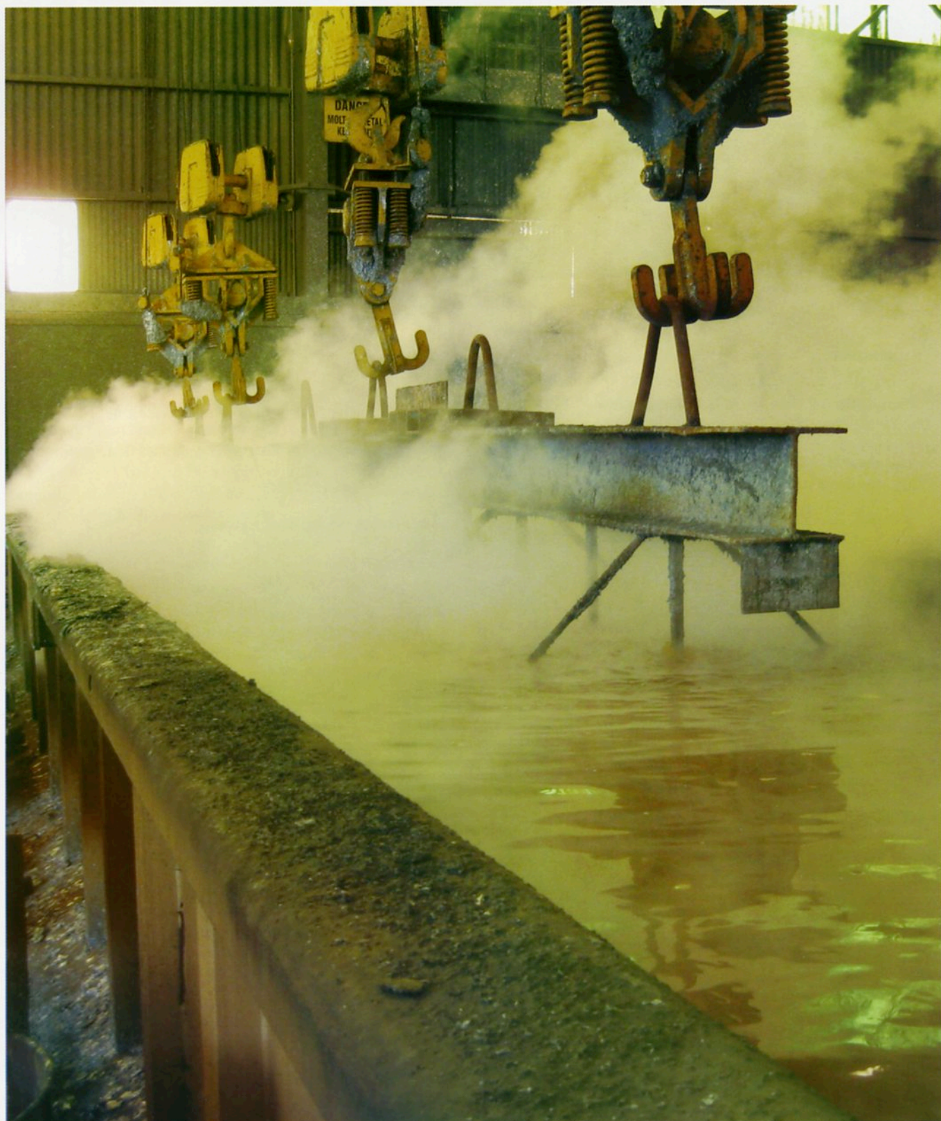
Much of the waste heat from the galvanizing process is recovered for heating process tanks and drying chambers.
