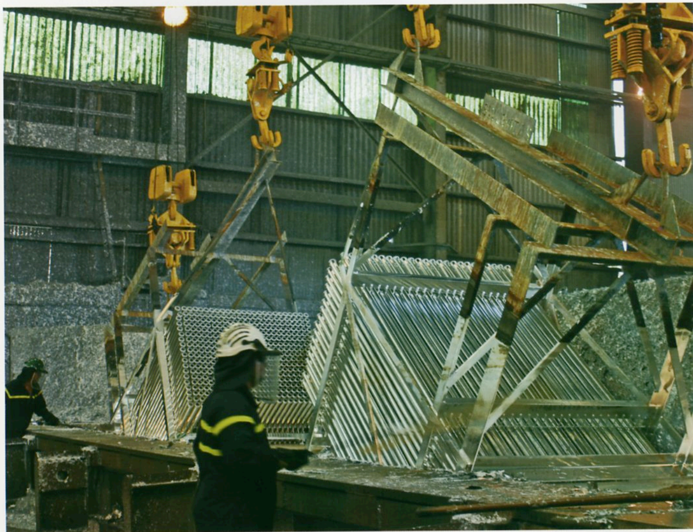
Hot dip galvanizing is a low-temperature process by metallurgical standards and has a relatively small carbon footprint.
