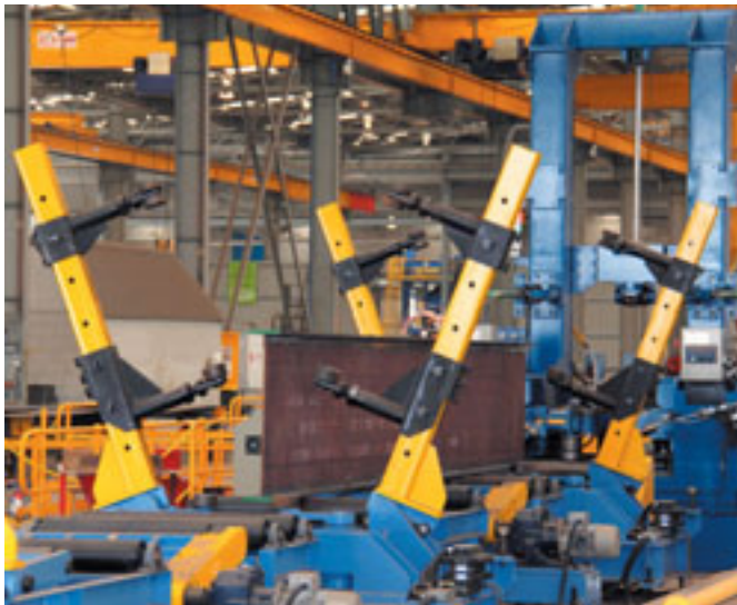
Samaras' Beam Assembly Welding and Straightening Machine.
