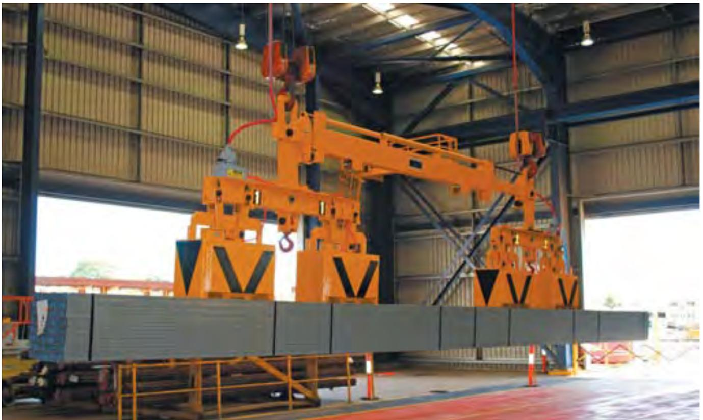
All the systems are capable of peeling off plate and pre-selection of the magnet force in order to speed-up picking operations and all the new magnet systems are controlled by HBC-radiomatic radio remote controls.
