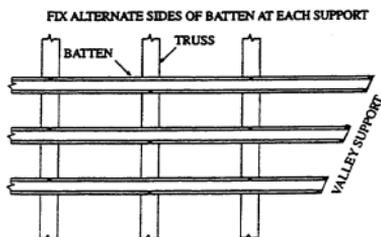
FIX BOTH SIDES OF BATTEN AT VALLEYS & HIP ROOFS
