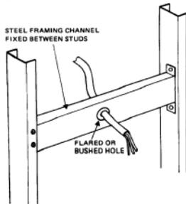
Wiring and Backing Plate
