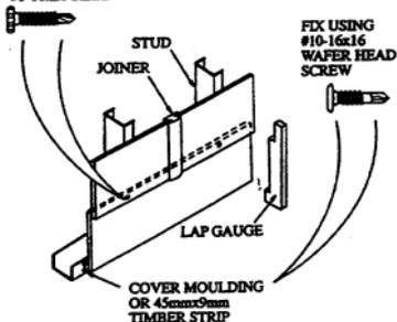
*Fibre Cement Fixing Details*
