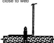
*Fixing Cladding to "C" Sections.*
