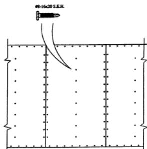
*Typical Fibre Cement Sheet Fixing Details*
