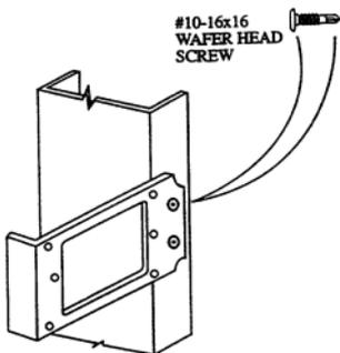
Switch & Power Point Backing Plate
