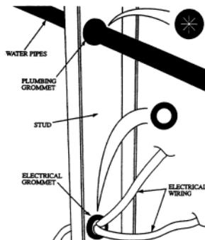
Installed Position of Electrical Grommets
