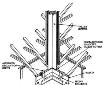
Typical Gutter Fixing, Valley Gutter in Place
