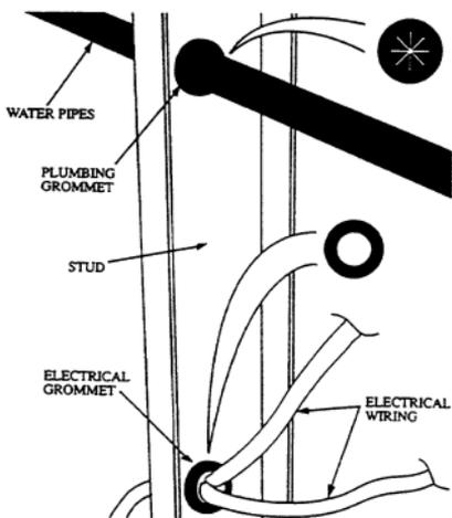
*Installed Position of Plumbing Grommets*
