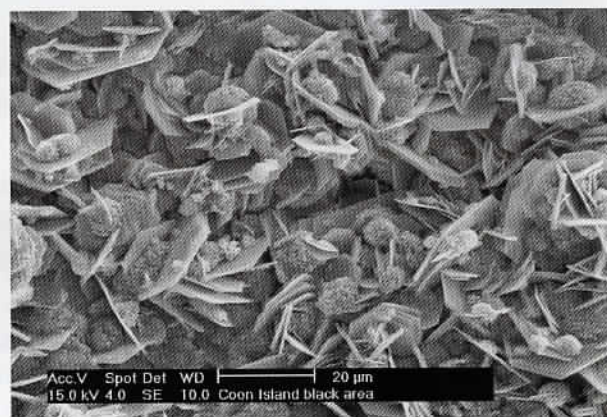
Figure 13 - Corrosion product showing tabular hexagonal crystals and 'spongy' globules.
