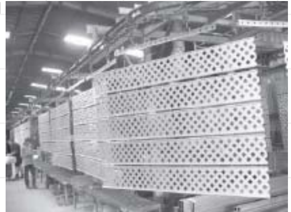
Polyester powder coating facilities have carefully controlled on-line pretreatment systems that ensure consistent surface preparation standards .
