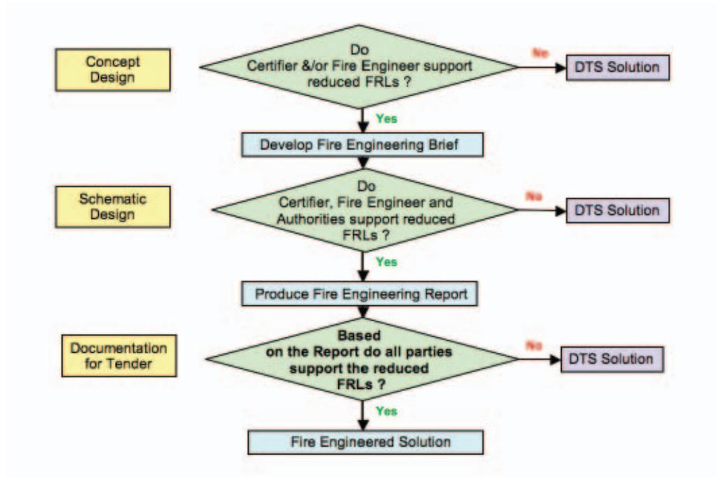
Figure 2: Alternate Fire Design
