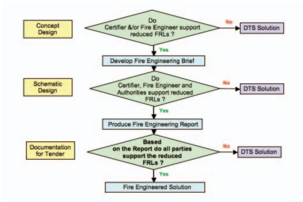
Figure 2: Alternate Fire Design
