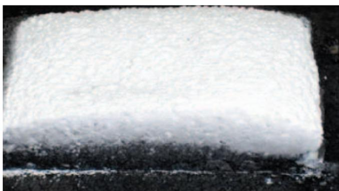
**Figure 9: Intumescent char insulating layer after fire**
