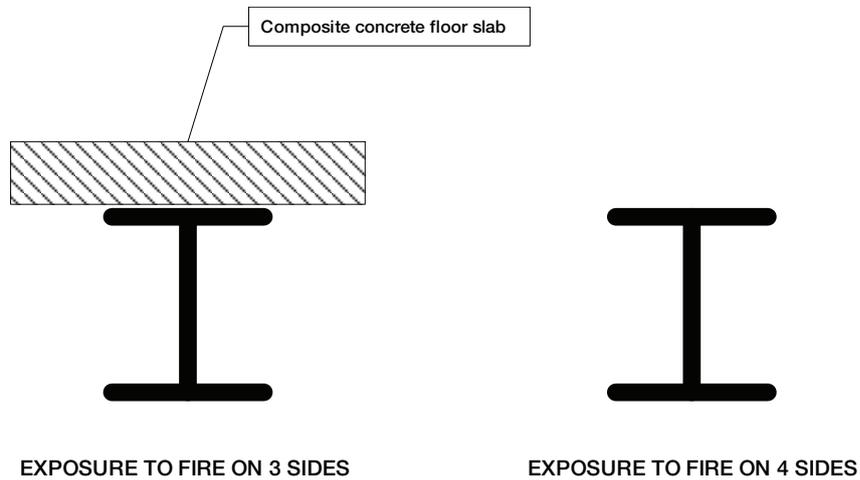
**Figure 1: Three sided and four sided exposure**
