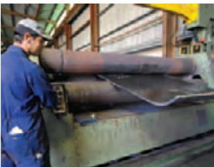
Wenco workers prepare XLERPLATE® steel to fabricate outer dome plate stove sections for the blast furnace maintenance project.
