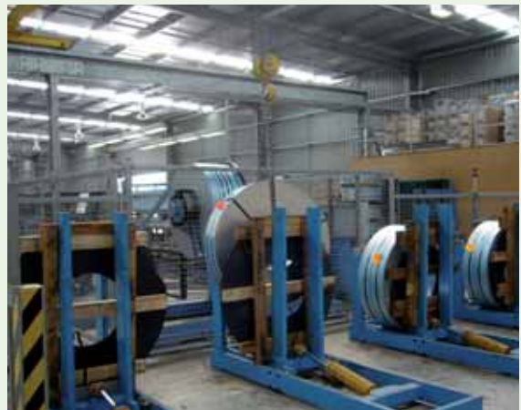
A purpose built device assists in moving heavy raw materials to the production line.
