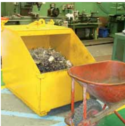
Readily available bin disposal with crane attachment for ease of emptying
