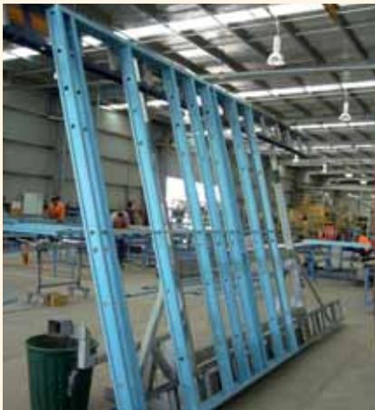
This jig enables the worker to assemble the frame in the best working zone.
