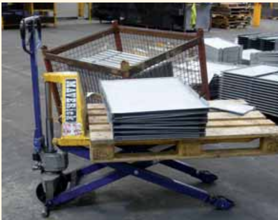
Pallet lifters raise products to best working zone.
