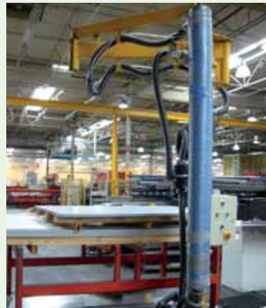
Vacuum lifter used to transfer material to machine table.
