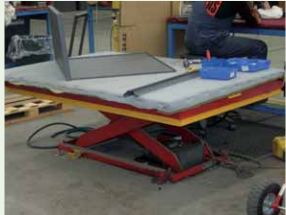
Hydraulic pallet lift table used as a workbench.
