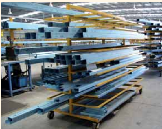
Trolleys used to transfer steel to the next workstation.
