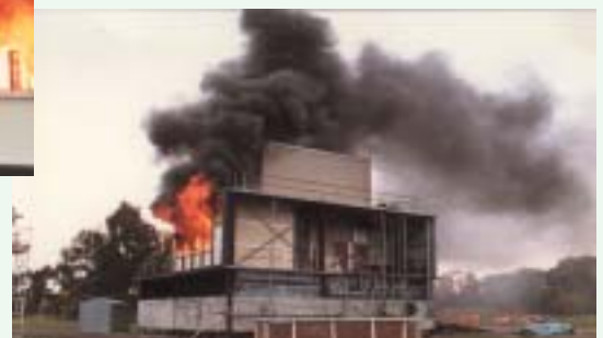
↙ view of test structure showing fire in office above imposed little threat to the carpark below
