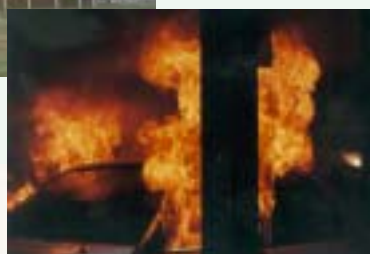
view inside test structure showing test vehicle alight
