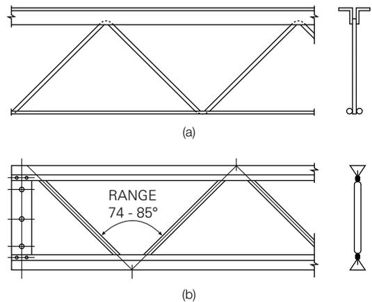
**FIGURE 8.23:** Types of open web joist
