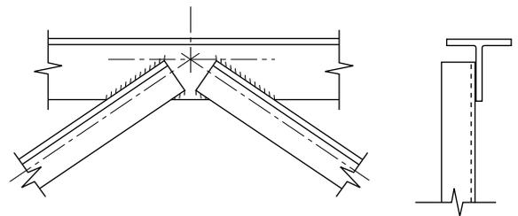
**FIGURE 8.20:** Split tee welded truss
