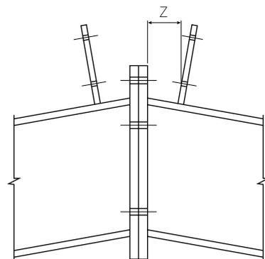
**FIGURE 8.25: Clearance at apex joint**
