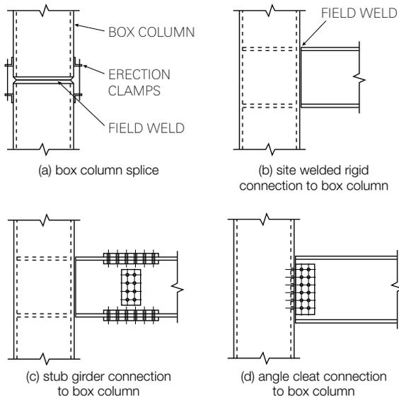
**FIGURE 8.16:** Connections to box columns
