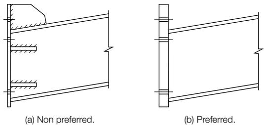
**FIGURE 8.24:** End plate details
