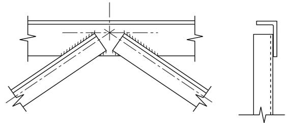
**FIGURE 8.19:** Single angle welded truss
