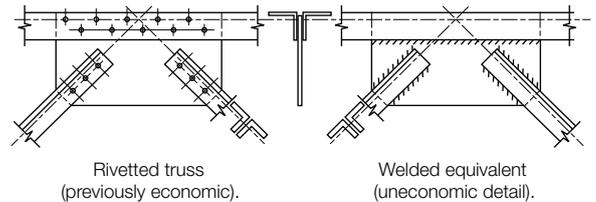
**FIGURE 8.18:** Equivalent truss detailing
