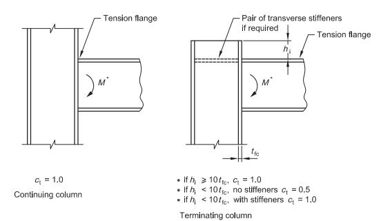
FIGURE 19 APPLICATION OF ct TERM—LOCAL BENDING AT TENSION FLANGE
