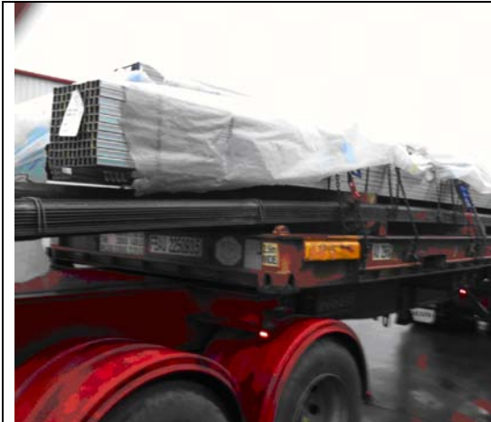
Inadequate tarping during local transport is a major cause of wet galvanized product and associated white rust.
