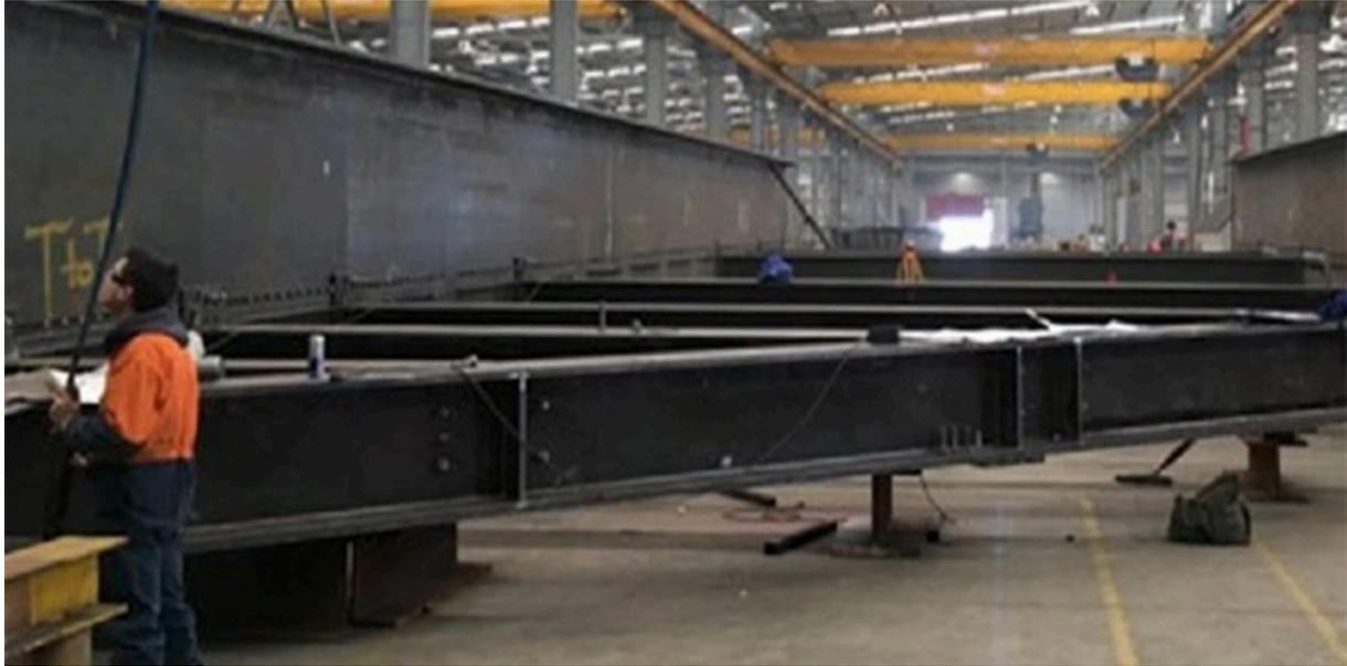
Fabrication is the process used to manufacture steelwork components that will, when assembled and joined, form a complete frame or structure. The frame generally uses readily available standard sections that are purchased from the steel manufacturer or steel distributor, together with such items as protective coatings and bolts from other specialist suppliers.
