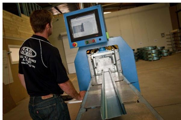
Roll forming machine operation. Image courtesy Enduroframe®.
