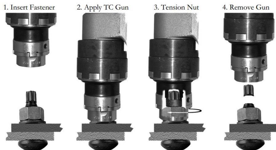
Figure 28 TCB wrench operation
