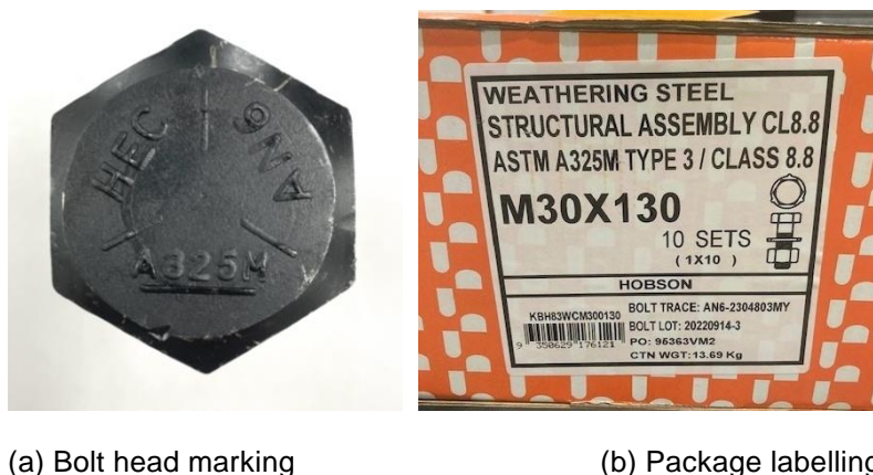
Figure 29 Example bolt head marking and package labelling for weathering steel bolt assemblies
