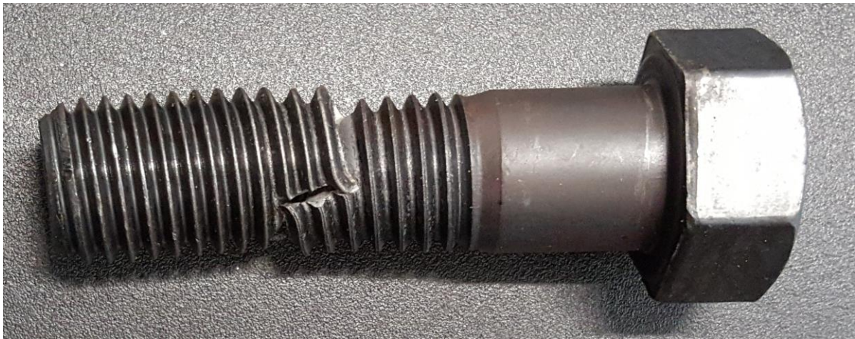
Figure B.4 Tension failure
