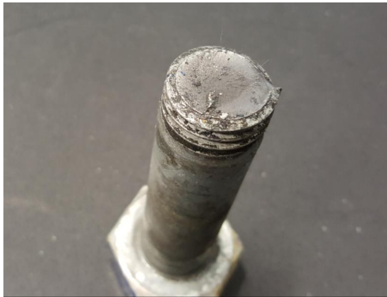
Figure B.2 Torque failure
