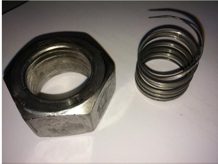
Figure B.5 Thread stripping failure
