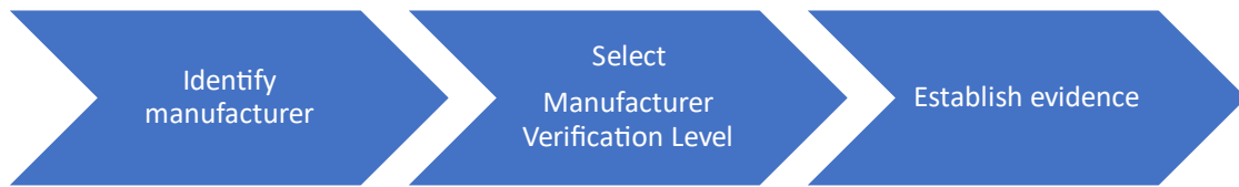
Figure 5 – Steel manufacturer verification process
