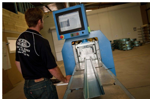
Roll forming machine operation. Image courtesy Enduroframe®.
