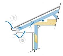
An eave with a small overhang may not contain a soffit lining. In this instance eave ventilation openings or devices may be provided at/or around the fascia (1b).
