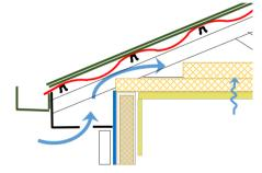
Impermeable reflective membranes are also used in combination with insulation blanket installed directly beneath metal roofing. The insulation blanket creates greater thermal insulation from the roof sheet, thereby affording protection against condensation in cooler climates.
