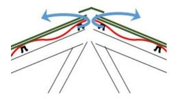
Practices that obstruct natural attic ventilation can lead to increased risk of moisture related issues in metal roofs. In this situation, additional ventilation should be considered.
