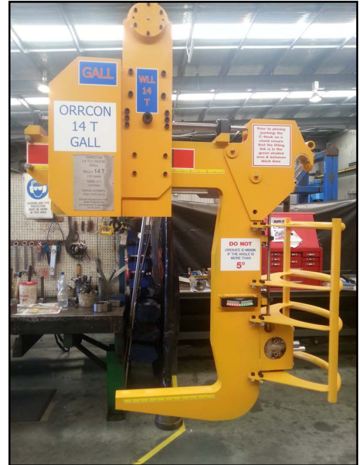
14T adjustable centre of mass C-hook
