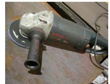
Angle grinder with guard removed and sanding disc attached.
