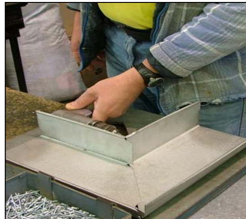
Figure 2 Drilling away from self - Preferred
