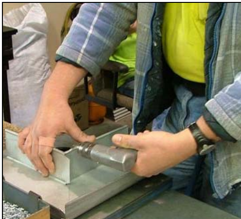
Figure 1 Drilling towards self – Not Preferred
