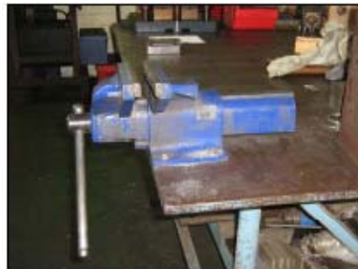
Above: Work should be secured in a vice, mounted on a bench at an appropriate work height.
