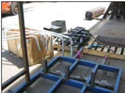
Above: work supported on wooden crate and pallets not facilitating an appropriate posture.
