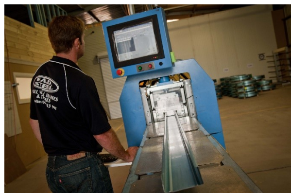
Roll forming machine operation. Image courtesy Enduroframe®.
