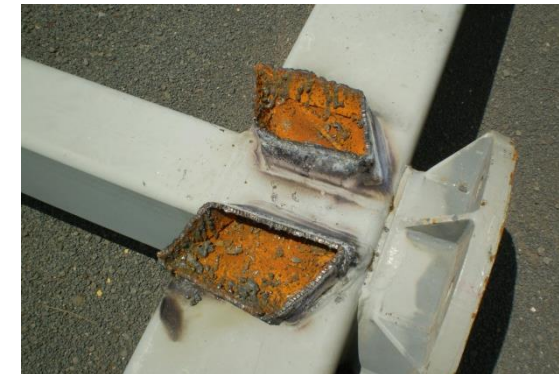
Wall thickness below specification
