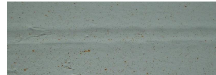
Under-cut (concave) weld below required thickness
