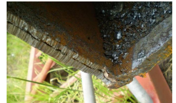
Fillet welded connection instead of butt weld
