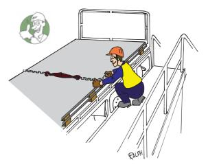
Use Platforms to attach load restraint and restrain load.
