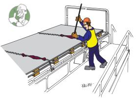
Tension chains using Platform for plate loads
